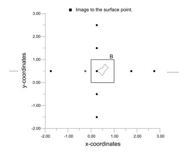
Figure 2. Image system for one point on the surface
